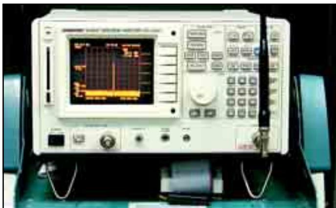
Figure 4—The Advantest R3361 spectrum analyzer used in the test.
